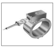
Quick-Disconnect Cup assemblies provide the simplest and safest means for applying power to any type of Cast-In Heater installation. The combination of prewired cup and box assembly, along with factory prewired high temperature lead wire protected with armor cable, eliminates live exposed heater terminals and electrical wiring, protecting employees from electrical shock and the possibility of electrical shorts due to exposed wiring.
