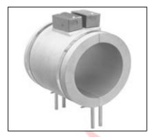
This is an individual terminal box for protecting the terminals on each Cast-In Band Heater half and on many other Cast-In Heater designs with one set of heater terminals. It is made from heavy gauge, rust-resistant sheet metal. The cover is removable for easy access to terminals. The box has two 7/8" diameter knockouts opposite each other for standard 1/2" BX connectors.
